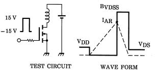
$\begin{array}{l} R_G = 25 \ \Omega \\ V_{DD} = 25 \ V\!\!\!, \ L = 428 \ \mu H \end{array} \qquad \qquad E_{AS} = \frac{1}{2} \cdot L \cdot I^2 \cdot \left( \frac{B_{VDSS}}{B_{VDSS} - V_{DD}} \right) \end{array}$
